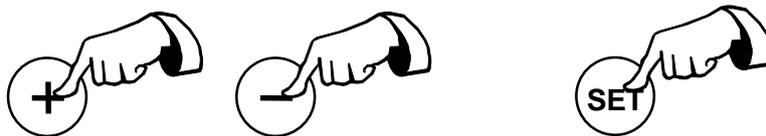
When pressing SET after setting the last parameter, the first parameter is shown again. To exit the parameter setting mode, press STOP or switch the machine off and on.
